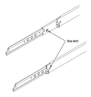
Figure 1-7: Installing or removing the rack slides
