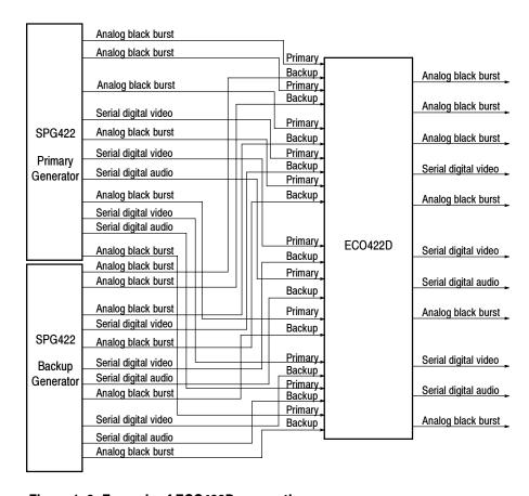
Figure 1-8: Example of ECO422D connections
