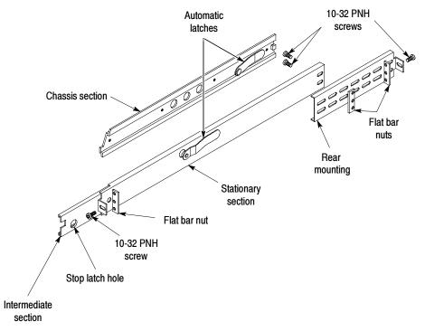
NOTE: Right hand and left hand stationary sections are designated by the RH and the LH markings on the rails. Stop latch holes should be toward the bottom when slides are in place. (The right hand rail is shown here.)
