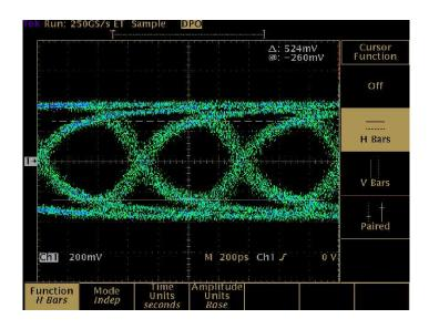
Figure 3-1: Typical eye-pattern of 20 m of Belden 1694A cable
