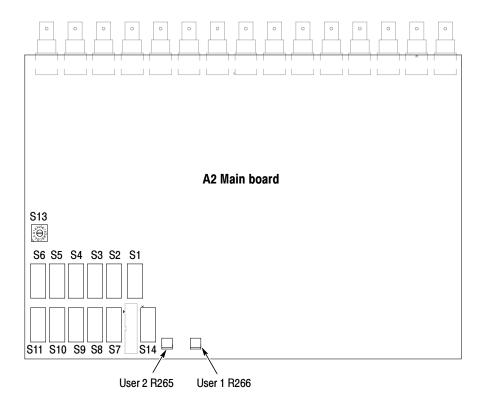
Figure 2-7: Selection switches and user level control locations
