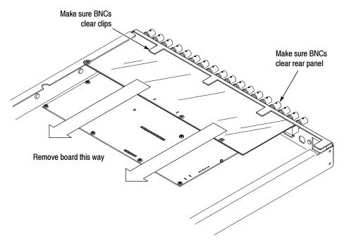
Figure 7-2: Slide the Connector board out this way
