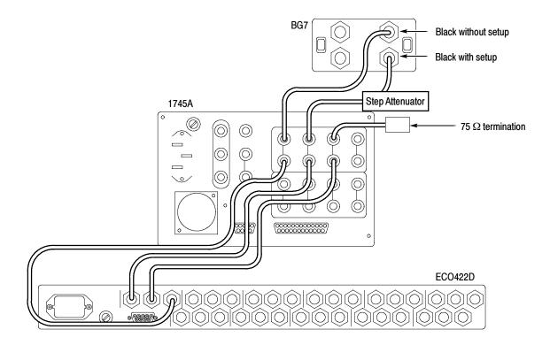
Figure 5-1: Setup to check Black Burst levels
