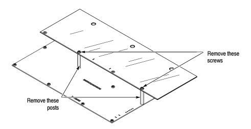
Figure 7-1: Remove these screws and posts before attempting to remove the Connector board
