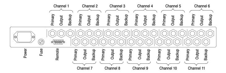
Figure 2-3: Rear panel of the ECO422D
