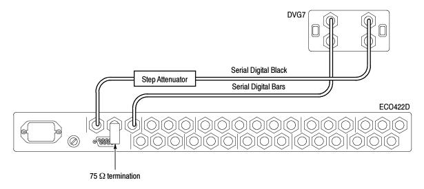
Figure 5-2: Setup to check the component serial digital video levels
