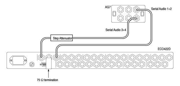
Figure 5-4: Setup to check the serial audio levels
