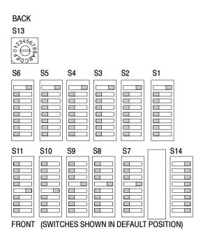
Figure 1-9: Default position of the User Configuration and Mode switches
