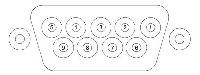
Figure 2-4: Remote connector pins
