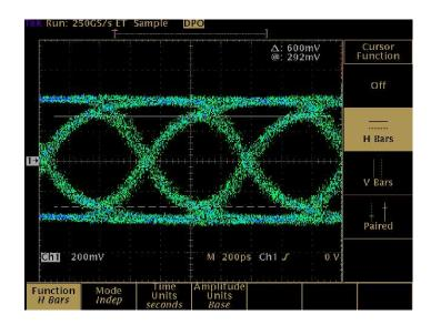
Figure 3-2: Typical eye-pattern of Channels 1-6 HD output (Channels 1-3 with Opt. ELSW)
