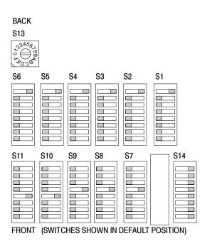
Figure 2-2: Default position of the user configuration and mode switches
