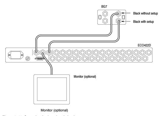
Figure 1-10: Setup for the functional check
